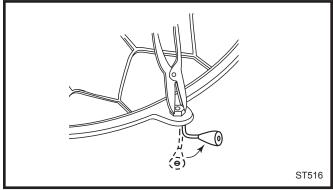
Fig. 17 Attaching the griddle handle.
